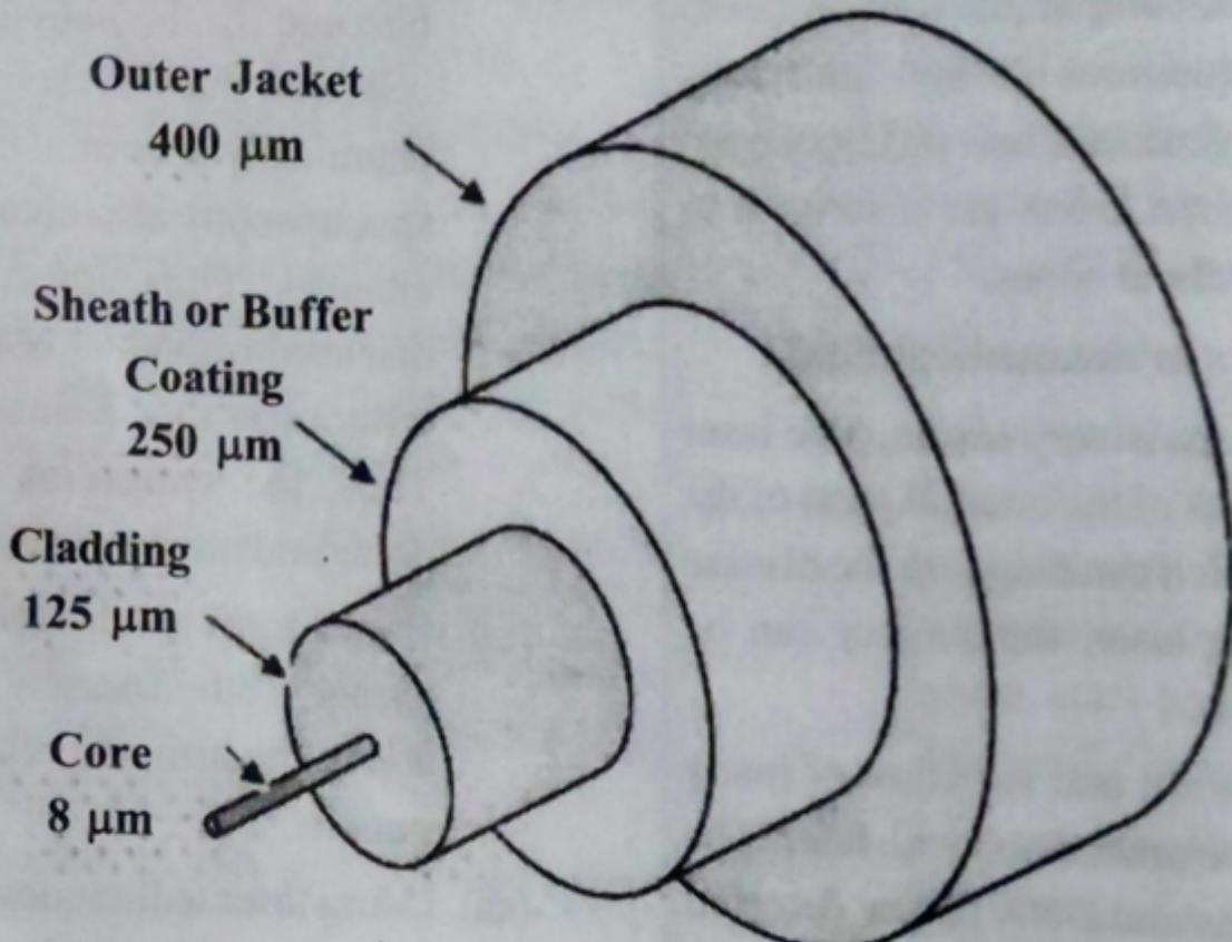
**Fig. 4.7 : Constructional Structure of Optical Fiber**
