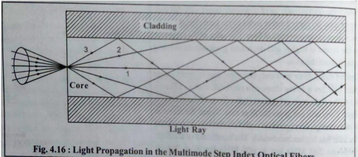
**Fig. 4.16 : Light Propagation in the Multimode Step Index Optical Fibers**
