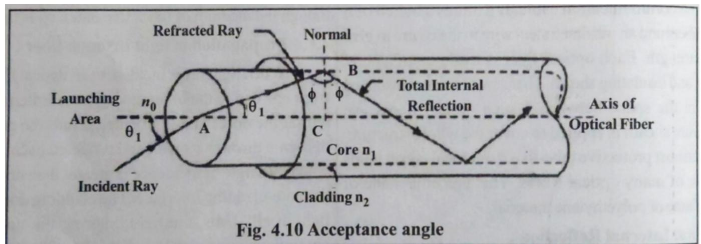
As shown in figure 4.10, light is incident at the launching end of an optical fiber.
